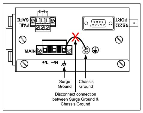
Figure 6 - Dielectric Strength Testing
